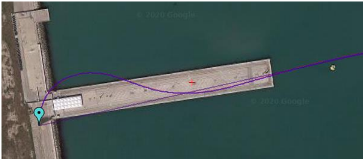
Figure 9-30: Transition between multirotor and fixed wing mode
